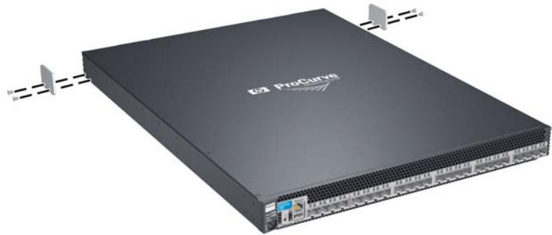
Figure 2-7. Installing the rail mounting holding brackets
